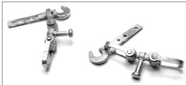
I pass the hook shank through the buffer beam slot then solder solid and trim off flush.
